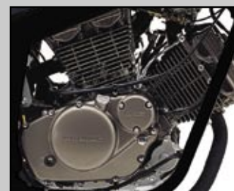
75° V-Twin DOHC engine
